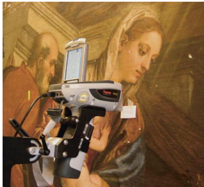
Colour pigments were determined using mobile X-ray fluorescence spectroscopy
